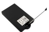
**Step 1**Separate the top from the bottom cover of the drive enclosure by loosening the screw as shown on the photo.
